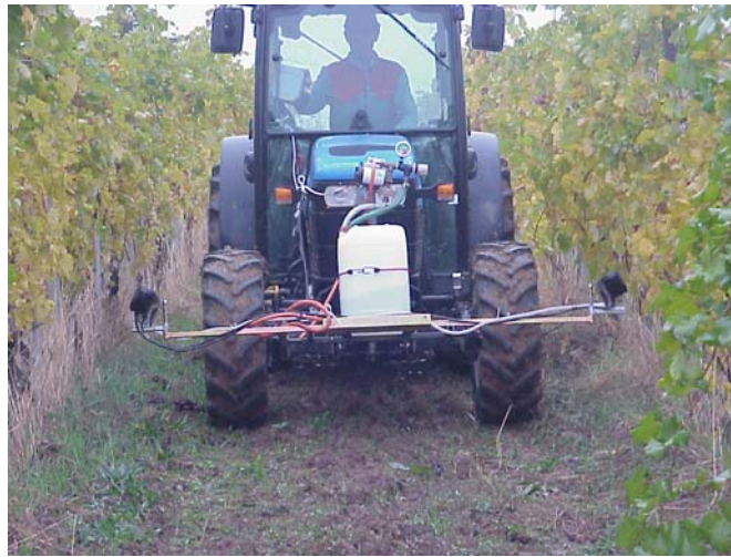
Figure 17 - Example of IR sensor used to detect the presence of weeds and to manage the spray application according to the infestation level detected.
