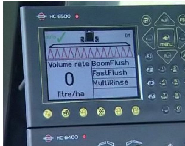
Figure 15 - Hardi Commander boom sprayer control panel equipped with the “Autowash” function enabling to manage automatically the complete internal sprayer cleaning.
