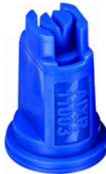
Figure 16 - Example of new air induction flat fan nozzle (Teejet AIXR03) featured by a reduced production of very small droplets (the percentage of droplets < 200 \mu m size is less than 1%; D10 = 290 \mu m; D50 = 567 \mu m; D90 = 842 \mu m, operating at 3 bar pressure).
