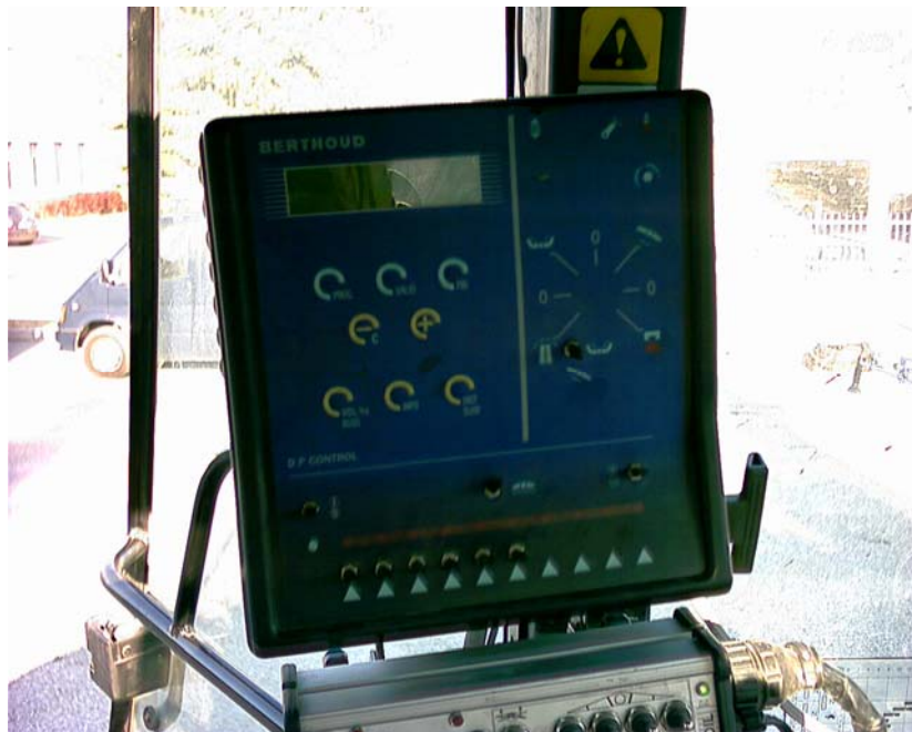
Figure 14 - Example of computer panel to check the actual applied volume. Source: [Berthoud].
