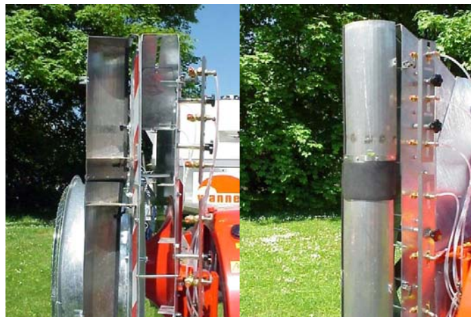
Figure 19 - Example of closing system of the air outlet on one side of an air-assisted sprayer.
