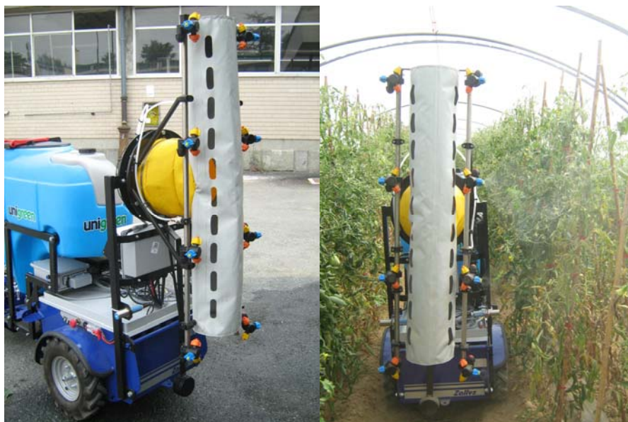
Figure 30 - Prototype of automatic sprayer to be used in greenhouses developed at DEIAFA University of Torino.
