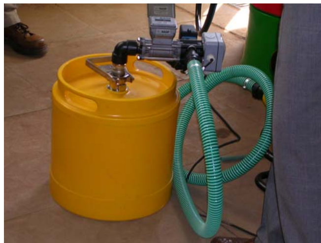
Figure 11 - Example of a PPP closed transfer system to introduce chemicals in the sprayer main tank.
