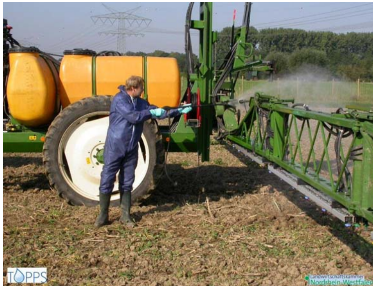
Figure 13 - Example of external cleaning of sprayer carried out using a spray lance. Source: [TOPPS].
