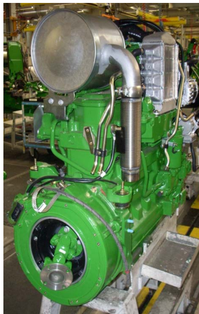
Figure 2 - Crankshaft mounted generator. Source: [3]
