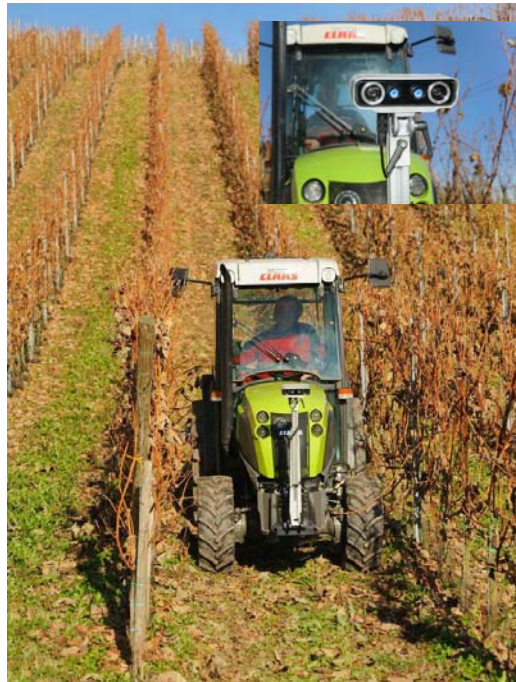
Figure 14 - The VineScout from company Clemens, [12]. The Vinescout guides vineyard tractors along the narrow tracks of vineyards.
