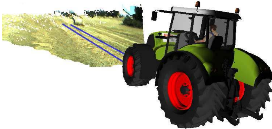
Figure 13 - Tractor auto-guidance system. The lateral and angular deviation between the field structure and the tractor is provided by the camera. A control signal is generated for the hydraulic steering system. The main components of an auto-guidance system are shown below. The system controls the front wheels while the driver controls the throttle and brakes and implement settings.
