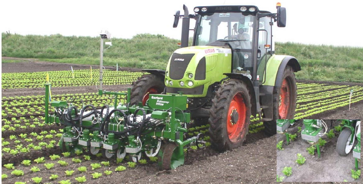
Figure 8 - RoboCrop InRow – complete inter-row and inter-plant weed control system from Garford [5].
