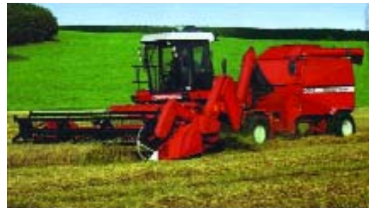
AZR-10 combine grain harvester “Polesje-Rotor” with front mounted header and axial rotary thresh drum-separator also attached behind to UES by the block of air-cleaning with a grain bunker. productivity on a grain up to 20 t/hr
