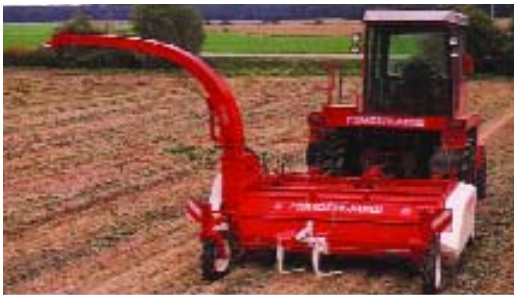
Sugar-beet harvester ASN-6 “Polesje” for one pass cuts tops, digs out, cleans and stacks roots in a row between wheels of power unit. productivity up to 2 hectare/hr
