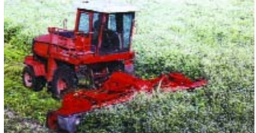
Rotary mower-crusher APR-6 “Polesje” with detachable conditioners for crushing of grass and stacking two swaths. productivity up to 6 hectare/hr
