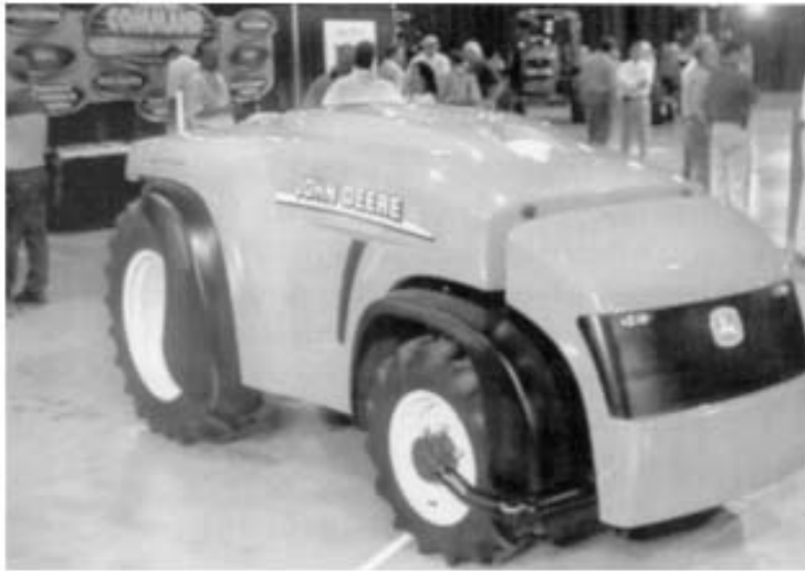
Figure 2 - The John Deere “driverless” orchard tractor has been publically presented in 2001. This type of tractor is intended to safely apply chemicals without operator assistance
