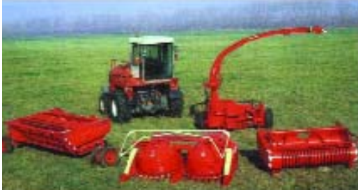
Forage harvester complex A-G-6 “Polesje” with chopper and adapters for cutting green grass, haying and silage from grasses and corn. productivity up to 90 t/hr
