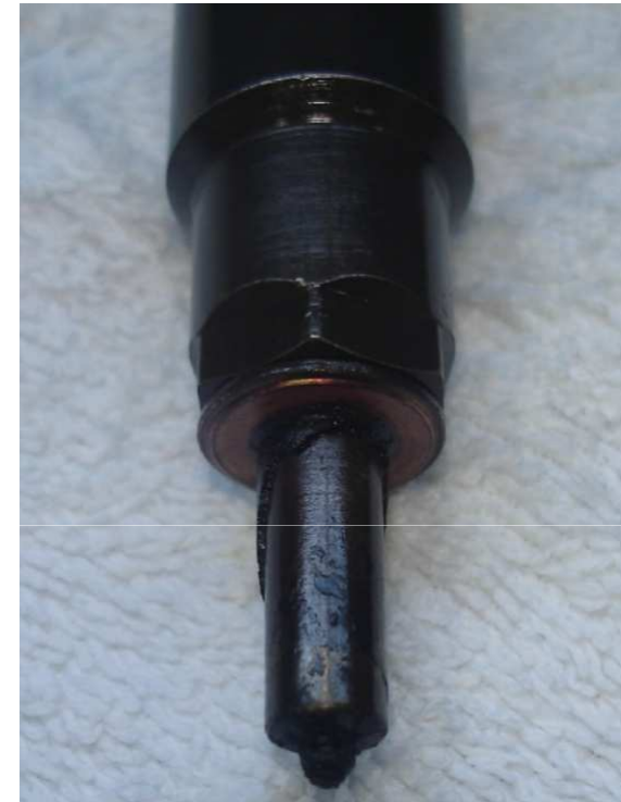
Damaged standard injector
