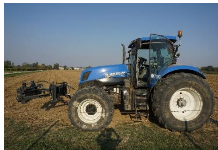
Fig.1b: Image of one of the tractors used in the validation tests. On the front of the vehicle is possible to see the device used to vary the mass distribution ( K_M ).
