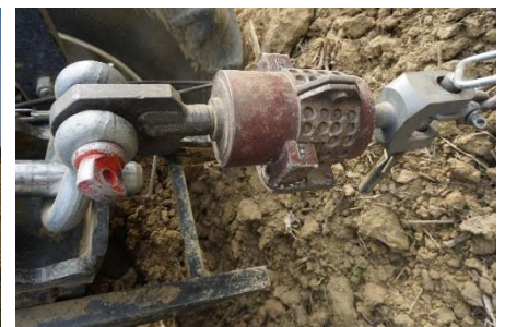
Fig.1c: Detail of the load cell used for the measurements of the drawbar force ( F_{DP} ) exerted by the tractor.
