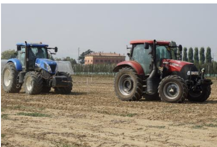
Fig.1a: Drawbar tests for the validation of the vehicle model under operational conditions. The rear tractor is used to exert a drawbar force on the front tractor, which is the one under test.
