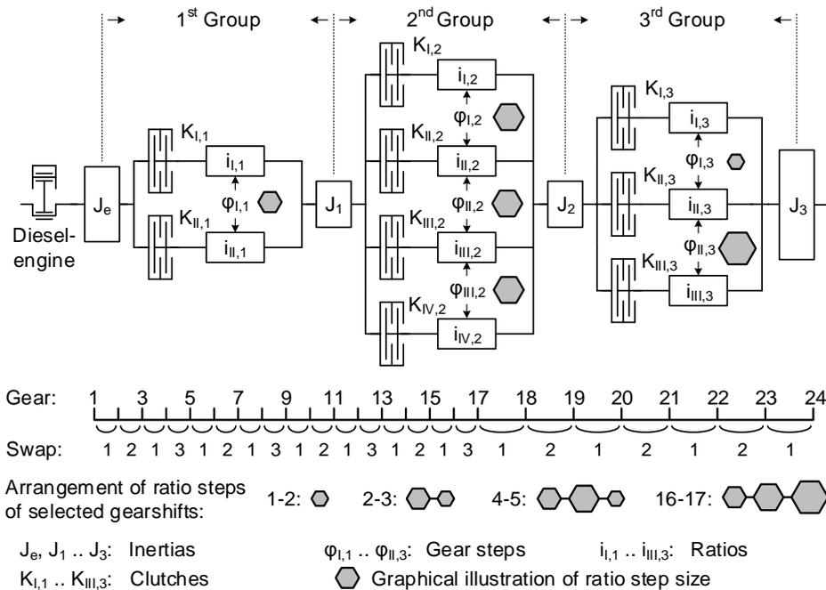
Figure 1: Transmission design and arrangement of ratio steps of an exemplary multi-group transmission
