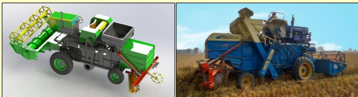
Figure 1 CAD model and field evaluation of developed seeding attachment
