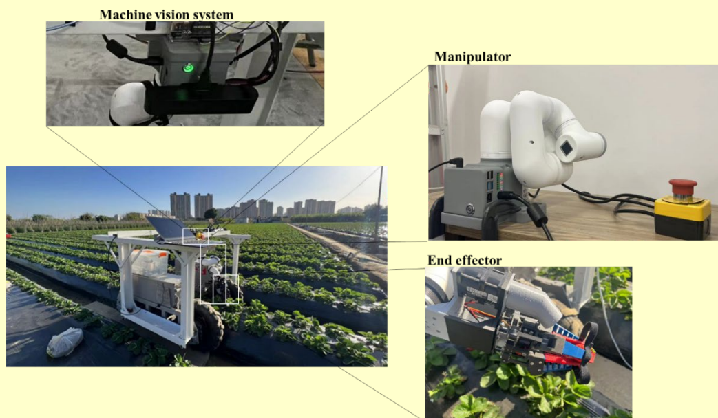
Figure 2. Robotic strawberry harvester including a machine vision system, manipulator, end-effector, and a ground platform.
