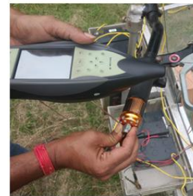
Fig. Measurement of vibration
