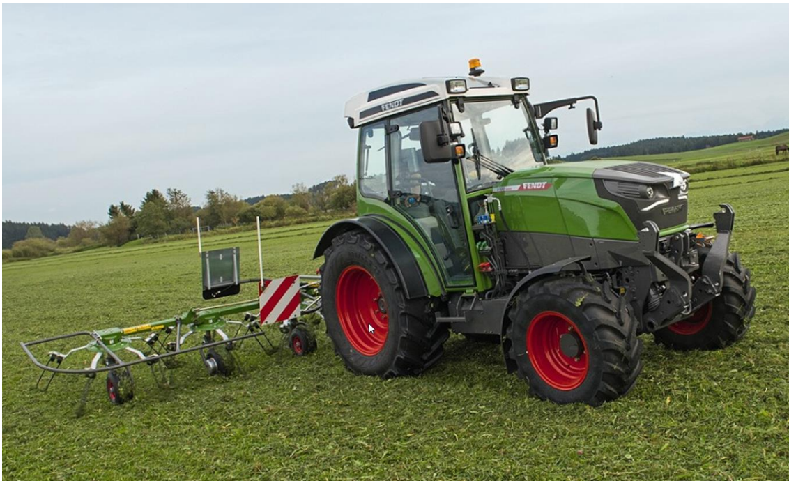
Figure 4 - The AGCO / Fendt e100 battery electric utility tractor with 50 kW rated power and a 100 kWh li-ion battery pack.
