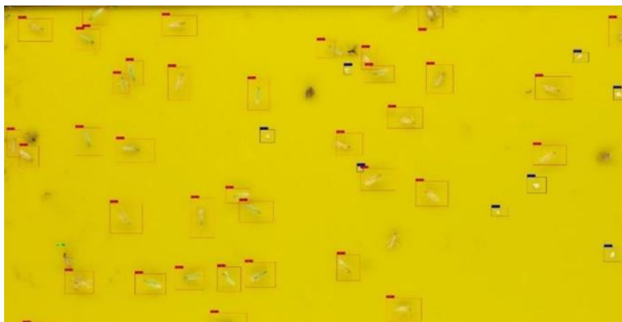
Figure 2 - Example results for automatic insect detection and counting on a yellow sticky trap. Source: [4].
