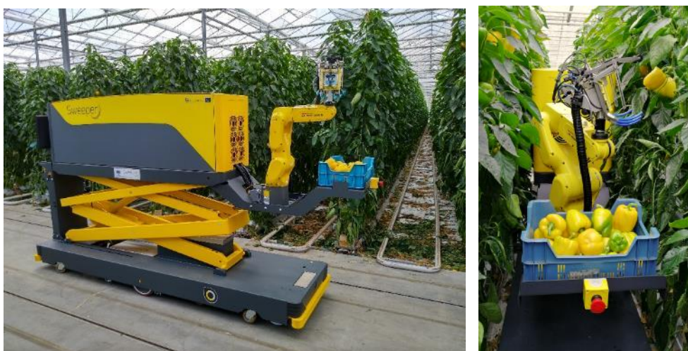
Figure 4 - The final prototype of the SWEEPER sweet pepper harvesting robot. Source: [9].
