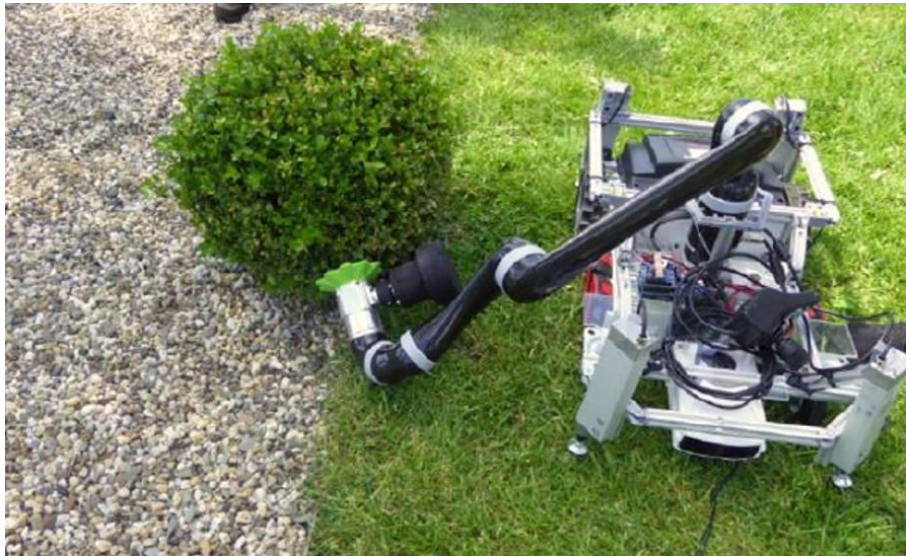
Figure 6 - Trimbot mobile platform with Kinova robot arm and bush trimming tool.
