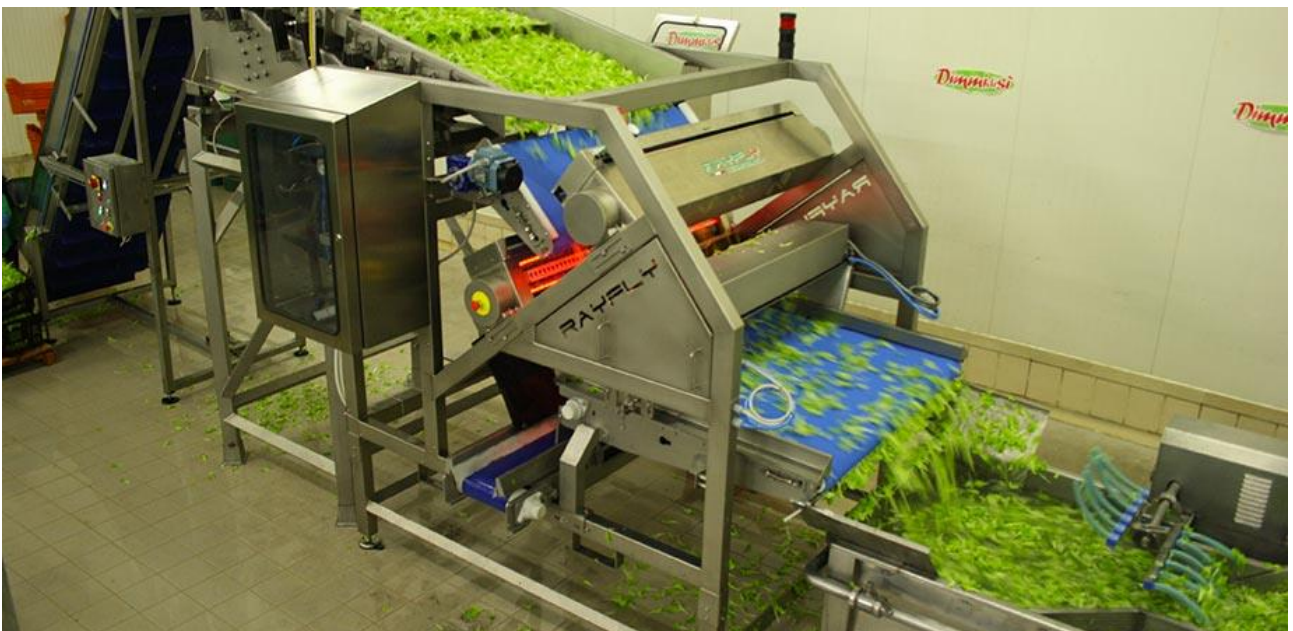
Figure 2 - Foreign body sorting machine on a ready-to-eat baby leaf processing line.
