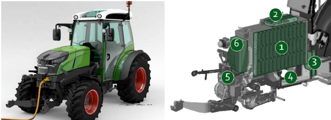
Figure 9: battery electric tractor Fendt e100 Vario [left] and basic feature concept [right: 1 - high-performance battery: 700 V, 100 kWh Li-Ion; 2 - DC quick charging and 400 V standard charging; 3 - efficient electric motor with high power density; 4 - dynamic power management; 5 - power supply for implements; 6 - innovative thermal management with heat pump] ( source: Fendt / Agco at Agritechnica 2017, Hanover)
